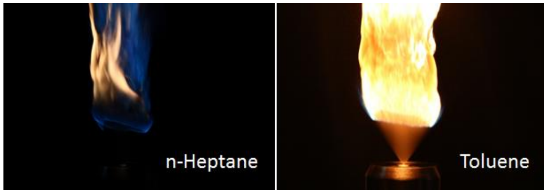
Figure 1.3. Flame images of n-heptane and toluene at 50 mL/min and 200 L/min fuel and air flow rates, respectively.
