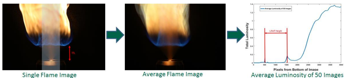
Figure 2.3. Liftoff height measurement procedure.
