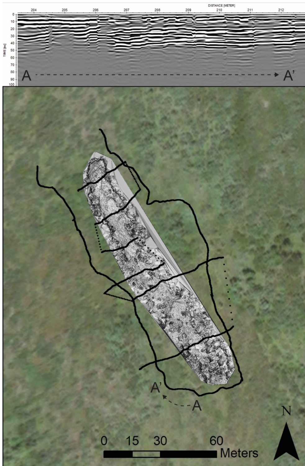
Figure C1. Example radargram and radar transect lines at the Ptarmigan ALD. GPR lines are overlain on a slope map derived from a TLS survey of the landslide conducted in summer 2018.
