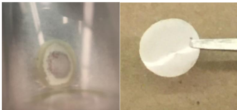
Figure B11: Left: representative digital photograph of a discolored polypropylene separator from a disassembled half-cell containing a \text{Cu}_2\text{Sb} thin film electrode cycled in 1 M \text{LiClO}_4 in EC/DMC/DEC (1:1:1 vol) electrolyte with an upper voltage cutoff limit of 3.0 V vs \text{Li}/\text{Li}^+ . Right: representative digital photograph of a polypropylene separator recovered from a half cell cycled without VC for comparison.
