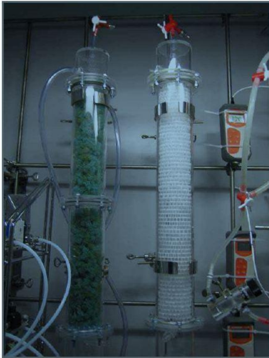
Figure 2-9 Bio trickling Filter for Siloxanes Removal (Ahrer, PROFACTOR, 2005)
