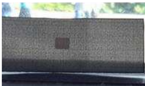
Figure 5.10: Attenuating masks placed in a window sill in order to demonstrate qualitatively the relative amounts of light passing through. The second attenuator which was printed “dark” across the whole mask and then a square piece of duct tape placed over the center in order to better block the light.
