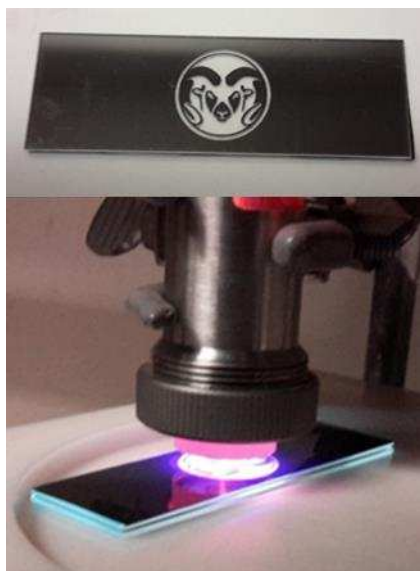
Figure 5.8: (Top) Glass slide, HA-FM swollen hydrogel and attenuator assembly. (Bottom) UV light source used to photopattern HA-FM into TPE hydrogel.
