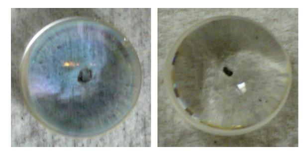
Figure 40 – Damage to focusing lenses in optical spark plug. Left: AR coated Gradium lens, sustained noticeable damage within 45 minutes. Incident beam was 9.2 mJ, 25 ns, ≈ 4.7 mm in diameter. Right: Uncoated SF11 lens, sustained noticeable damage within 2.5 hours. Incident beam was 9.2 mJ, 25 ns, ≈ 7.0 mm in diameter.
