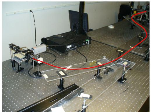
Figure 17 – Configuration (c), "?" shape. Fiber highlighted in red. Final bend  $\approx 40$  cm radius of curvature.
