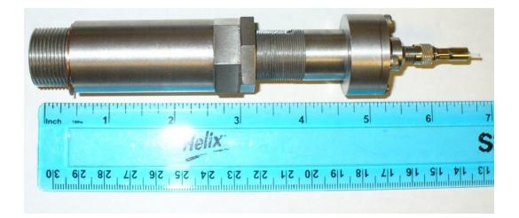
Figure 21 – Assembled optical spark plug.
