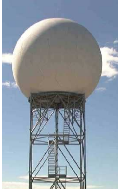
FIGURE 3.2. Picture showing a next generation weather surveillance radar system. The white round ball shaped enclosure is the radome which is supported by mechanical structure. The radar is located within the radome. Image source: https://www.roc.noaa.gov/WSR88D/Engineering/NEXRADTechInfo.aspx
