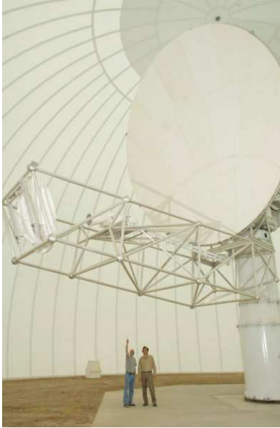
FIGURE 3.3. Picture showing CSU-CHILL radar inside the radom enclosure at the CSU-CHILL National Radar Facility. Image source: http://www.chill.colostate.edu/w/Facilities
