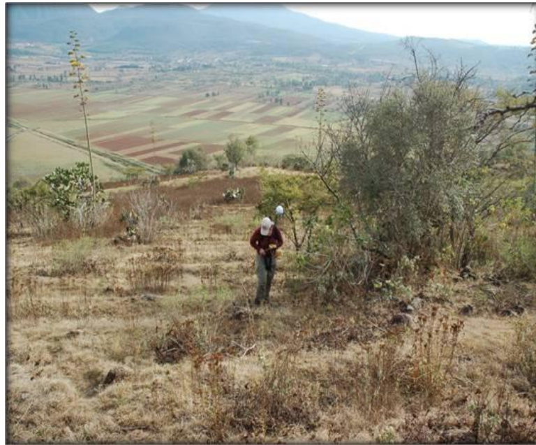
Fig. 5.6. Surveying Apúpató with sub-meter accuracy DGPS running Tripod Data Systems(TDS) Solo Field software and real time correction (Omnistar)
