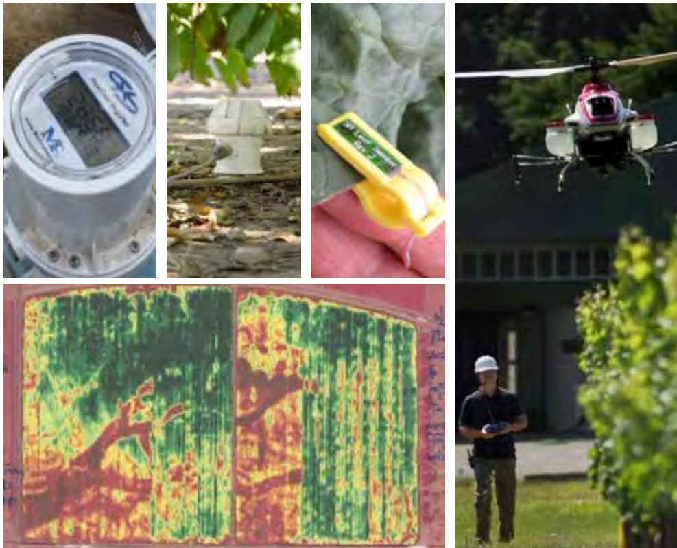
(Clockwise from top left) water meter, soil moisture probe, direct leaf monitoring, drone helicopter, and remote sensing image. Photos courtesy of David Zoldoske.
