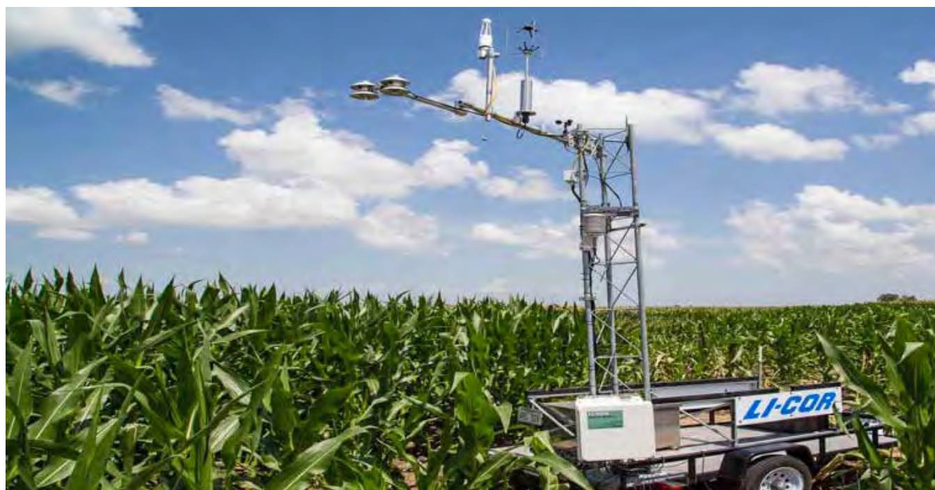
Figure 3. Mobile eddy covariance flux tower positioned in a cornfield near Brule, Nebraska, running SmartFlux2 and connected with FluxSuite. Photo by Dayle McDermitt, LICOR Biosciences, Lincoln, Nebraska.
