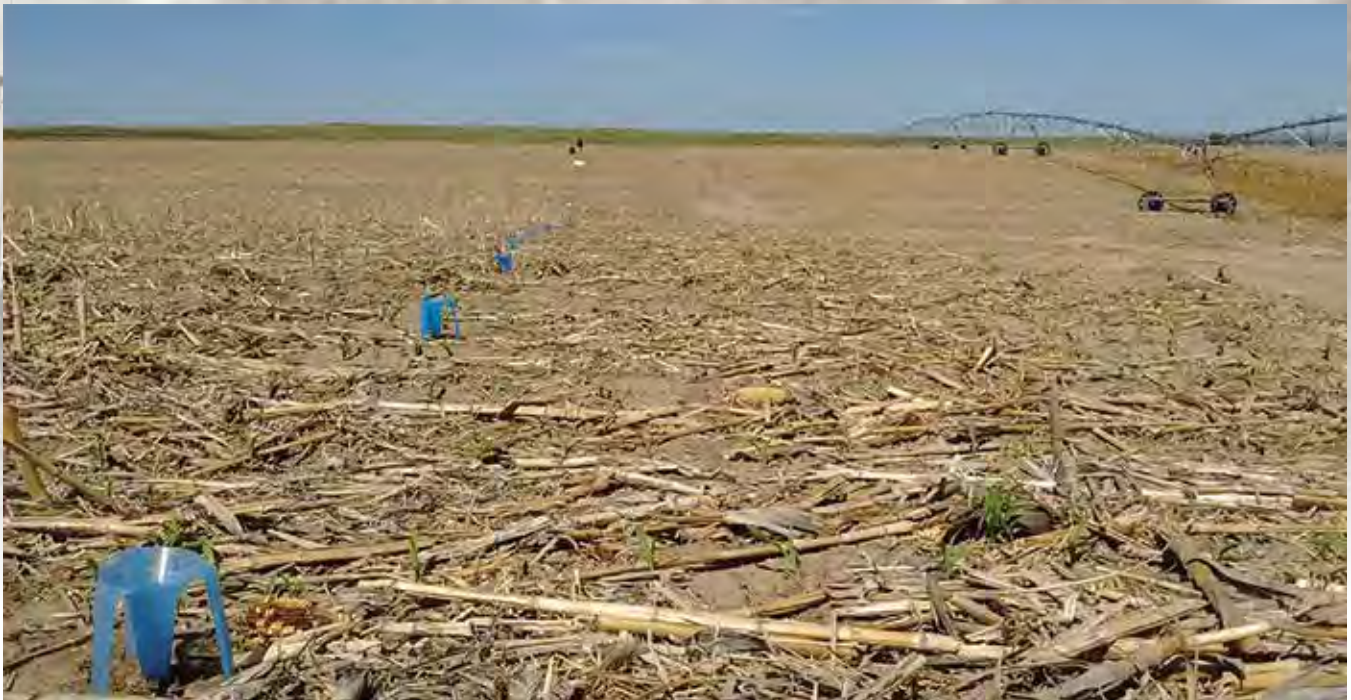
Variable rate irrigation system and catch cans at the Brule field site. Photo courtesy of Sandeep Bhatti.
