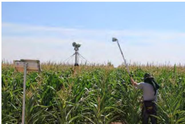
Figure 3. FLIR Tau2 LWIR (top), Tetracam Mini-MCA6 (bottom). Photos courtesy of Dr. Huihui Zhang
