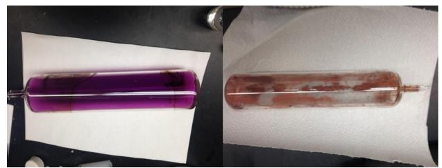
**Figure 1-3.** Side-by-side ampules charged with  $CF_3I$ . (Left) No  $Cu_{(s)}$  was added. (**Right**)  $Cu_{(s)}$  was added. The two ampules were heated to allow  $CF_3I$  bond dissociation to occur and the resulting images show the effect Cu(s) powder has on  $I_2(g)$  formation. At no point during the test was visible  $I_2(g)$  formed in the  $Cu_{(s)}$  containing ampule.
