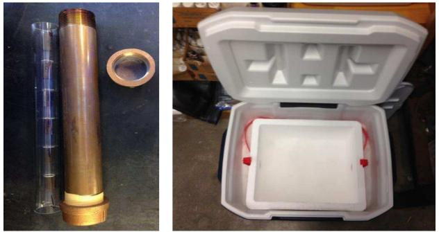
**Figure S4-1.** (Left) Air-tight vessel for thermal cycling of OPV active layers. The glass tube shows the arrangement of the slides inside the chamber. (**Right**) Low temperature chamber, -78 °C. High temperature chamber, 100 °C, was a lab grade oven.
