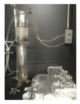
**Figure S4-2.** 450 W high-pressure mercury-arc lamp for UV radiation exposure tests. The films were placed along the aluminum wrapped lead brick to minimize the variation in exposure based on position for the films.
