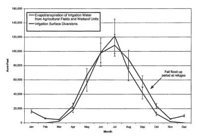
Figure 4. Irrigation surface diversions and the evapotranspiration of irrigation water from agricultural fields and refuge wetlands in the Klamath Project area of investigation (avg. of 1999-2000). [Vertical bars indicate confidence intervals of data ]
