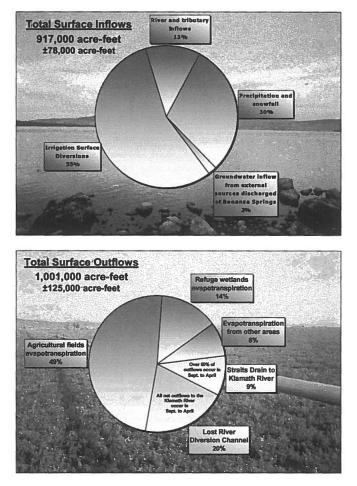
Figure 3. Surface water balance of the Klamath Project (avg. of 1999-2000)
