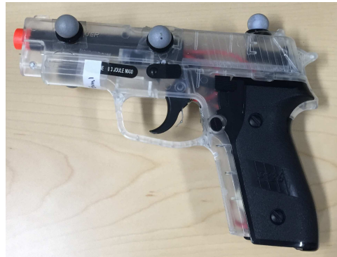
Figure 4. The laser gun used for Experiment 2 with the reflective markers used for the motion tracking system.
