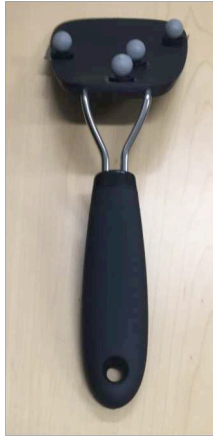
Figure 5. The spatula used for Experiment 2 with the reflective markers used for the motion tracking system.
