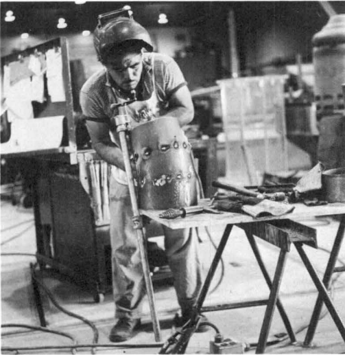
Fig. 6(c) Constructing reducing bend
