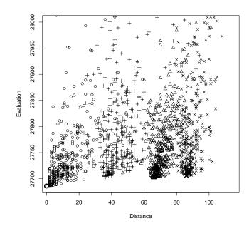
Figure 4.2: 500 local optima found by LK search when starting at each of the four funnel bottoms in att532. Each local optima is shown with a symbol matching the initial tour of the walk. The initial tour, i.e. the funnel bottoms, are shown with a slightly larger and bolder symbol. The initial tours have evaluations from left to right of 27686 (optimal), 27705, 27703 and 27706.
