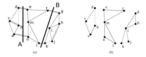
Figure 2.3: An example of (a) The graph G created from the union of two parent tours with two partitions of cost 2 shown by the heavy dark lines and (b) The graph  $G_u$ , constructed by deleting the common edges edges between the two parent tours from G
