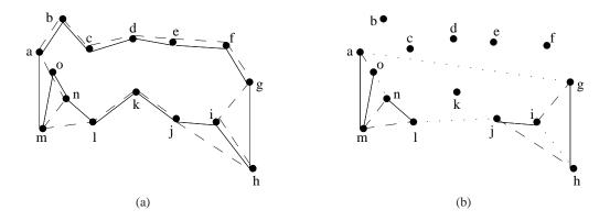
Figure 2.1: An example of (a) The union graph of two parent tours (one shown by solid lines, the other by dashed) and (b) The reduced graph  $G^*$  made by replacing common paths with surrogate edges (dotted lines).
