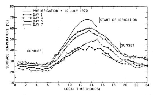
Figure 8. Diurnal Surface Temperature Variation as Measured by a Thermocouple. (Data from U.W. Water Conservation Laboratory in Phoenix, Arizona, Schmugge et al. 1978).
