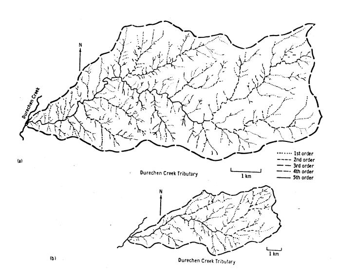
Figure 4. Correlation between drainage basin data derived from topographic map and from radar imagery of the Durechen Creek tributary. (a) Topographic map; scale of 1:24,000. (b) K-band radar. (Rouse and Molly, 1975)
