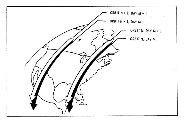
Figure B2. Landsat ground coverage pattern.
