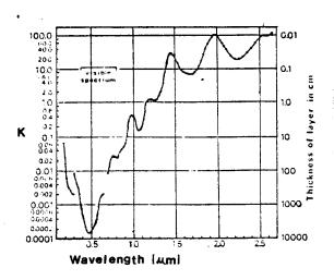
Figure 1. Absorption coefficient (K) for pure water, wavelength range 0.2 to 2.6 µm. (From Manual of Remote Sensing, Reeves, 1975).
