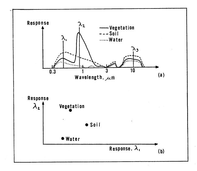
Figure A-2. Multispectral data may be presented in several ways. Figure (a) shows reflectance plotted as a fundtion of wavelength. Figure (b) shows spectral data in two-dimensional spectral space. (After Landgrebe, 1976).
