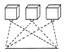
Full color images can be produced when each of the separate images is processed and superimposed in its respective color on a single frame. Technical malfunctions forced the RBV systems to be shut down shortly after launch. The RBC system of LANDSAT-3 is a modification of its predecessors. It includes two panchromatic cameras which generate two side-by-side images rather than superimposed images of the same target. This system has been returning imagery when requested since its launch in 1978.
