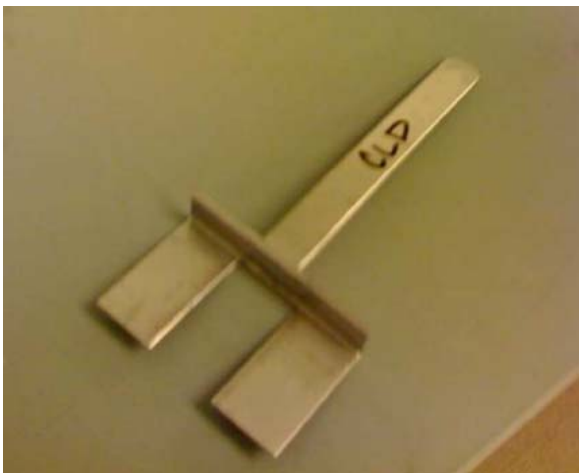
Fig. 4.8 The chip lifting device
