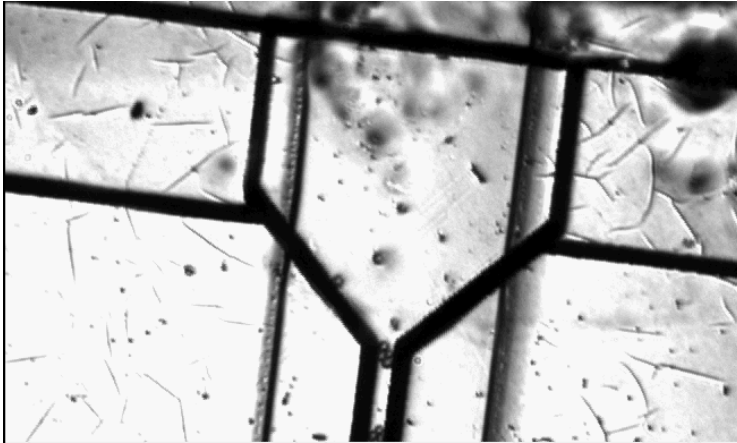
Fig. 9.2 A snapshot from video showing majority of the cells were being funneled.
