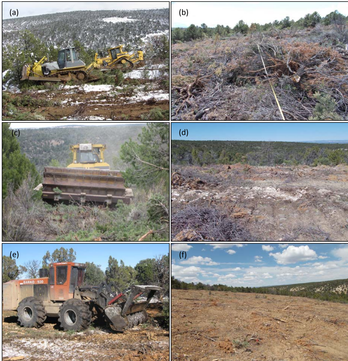
Fig. 1. Pinyon-juniper removal using different mitigation treatment methods (left photos) and examples of post-treatment conditions (right photos) in experimental plots cleared with a) chaining, c) roller-chopping, and e) hydro-axing. Chaining involves dragging an anchor chain connected to two tractors across a stand, toppling trees (a), and produces plots with abundant slash and small standing trees and shrubs (b). Roller-chopping involves dragging a heavy drum with attached blades behind a tractor; the weight of the drum crushes trees and brush, while the blade chops the slash (c), resulting in a bed of crushed slash and distinct soil disturbance patterns (d). Hydro-axing involves using a tractor with an articulating mulcher-head attached to the front that mulches stems < 8 inches in diameter (e). This technique produces a bed of fine mulch (f). Photo credits: Garrett Stephens (machinery) and Travis Gallo (plots post-treatment).
