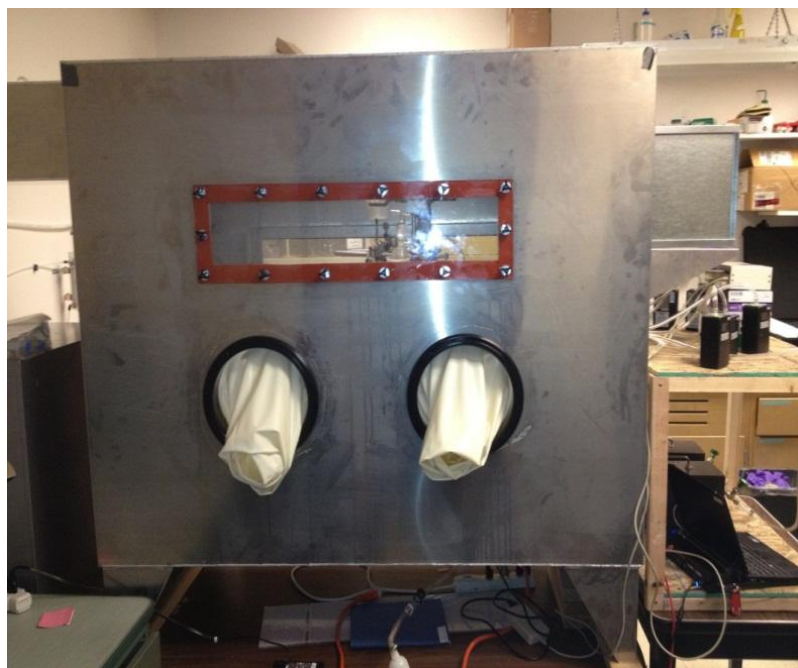
Figure 4.3.1: Schematic of the aerosol chamber and a picture of the aerosol chamber; adopted from John S. Frazey, Ph.D. Candidate.
