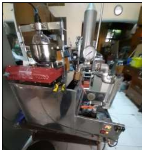
Fig. 2. The evaporator used to lower the moisture content in honey
