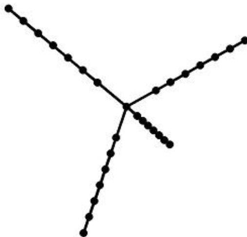
Figure 3.2 One-Dimensional Mesh of Tetrahedral Ligament Microstructure [25]
