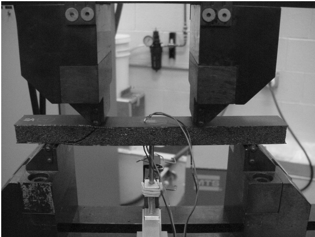
Figure 3.7 Initial Failure Due to Shear Stress in the Core (Specimen 4)
