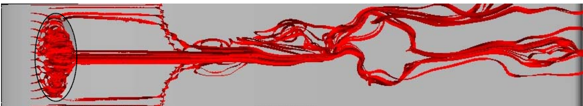
Figure 33. Enlarged view of CFD suction surface streamlines for a Pak-B blade with spherical dimples at 60% axial chord. The axial view shows flow from left to right
