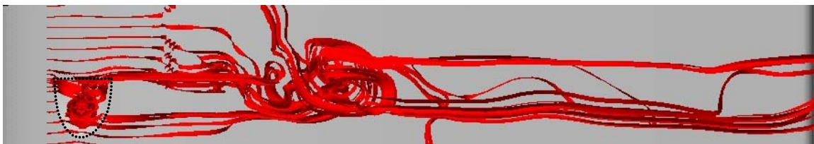
Figure 35. Enlarged view of CFD suction surface streamlines for a Pak-B blade with asymmetric dimples at 60% axial chord at Re 25k. The axial view is shown with flow from left to right
