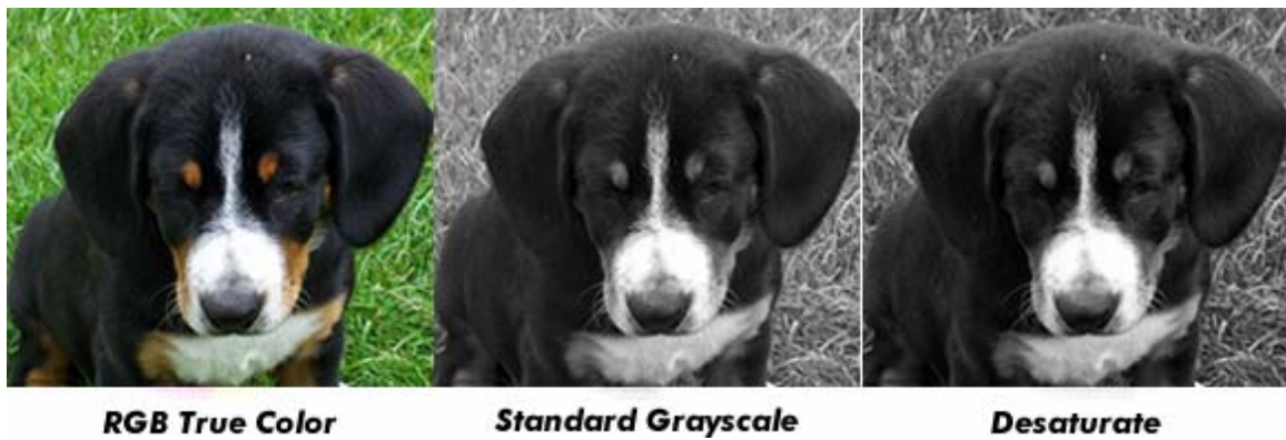
Figure 10. A Comparison of the Grayscale Functions on a True Color Image
