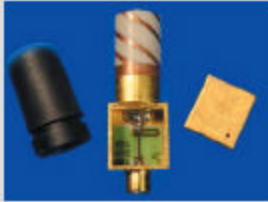
GeoHelix-P is a passive antenna
