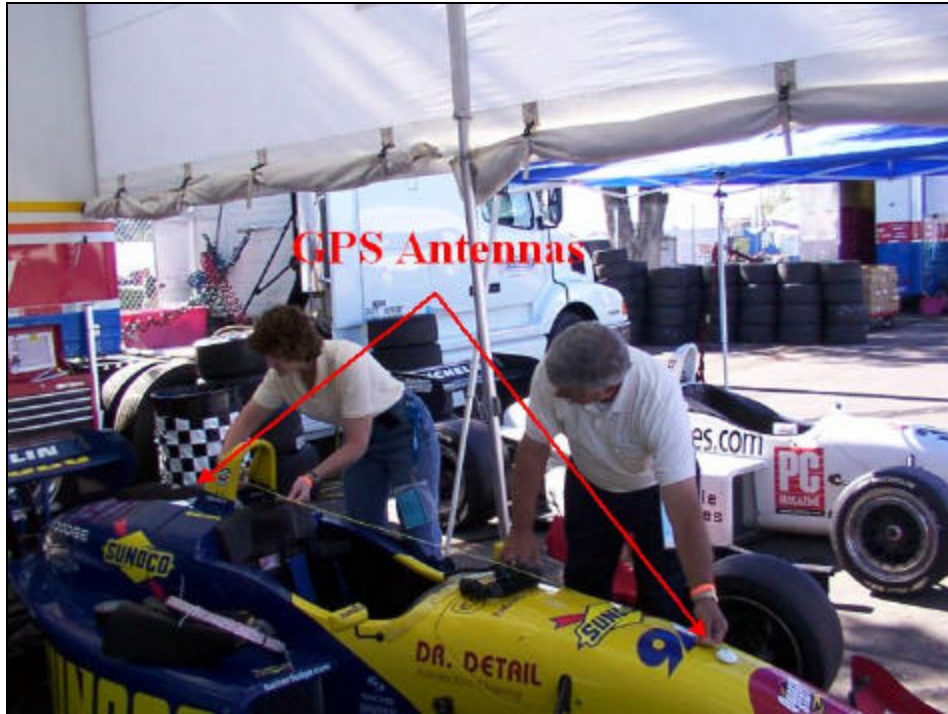
Figure 18. CART Antenna Placement
