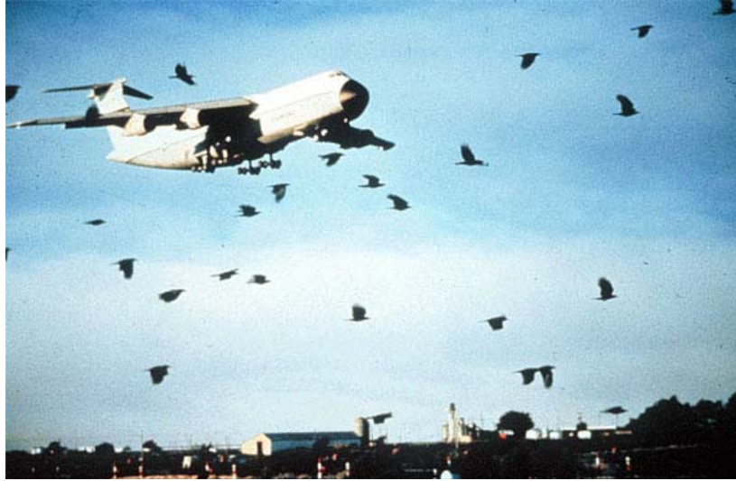
Figure 2-22: Bird Strike Hazard to C-5 (United States Bird Avoidance Model for Military and Civilian Pilots, 2002)
