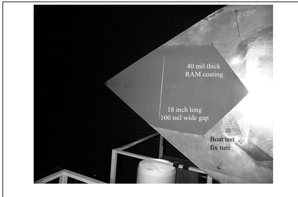
Figure D.5 The gap is located 22 inches back from the tip and 34 inches from the center of rotation of the boat fixture.
