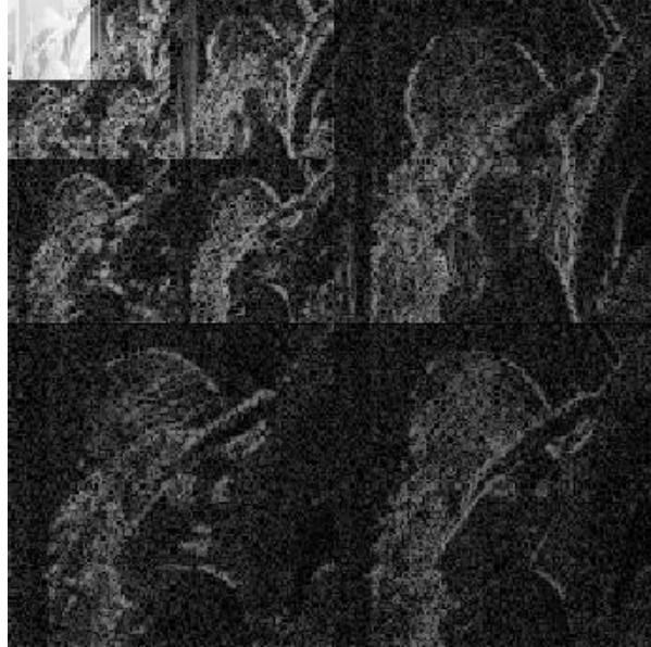
Figure 2.4: The original “Lenna” image after three iterations of the wavelet transform. The first iteration HH, HL, and LH subband are the same as before. The other iterations of the HH, HL, and LH subbands extract more information from the previous LL subband image. The final LL subband is an extremely coarse version of the original image.
