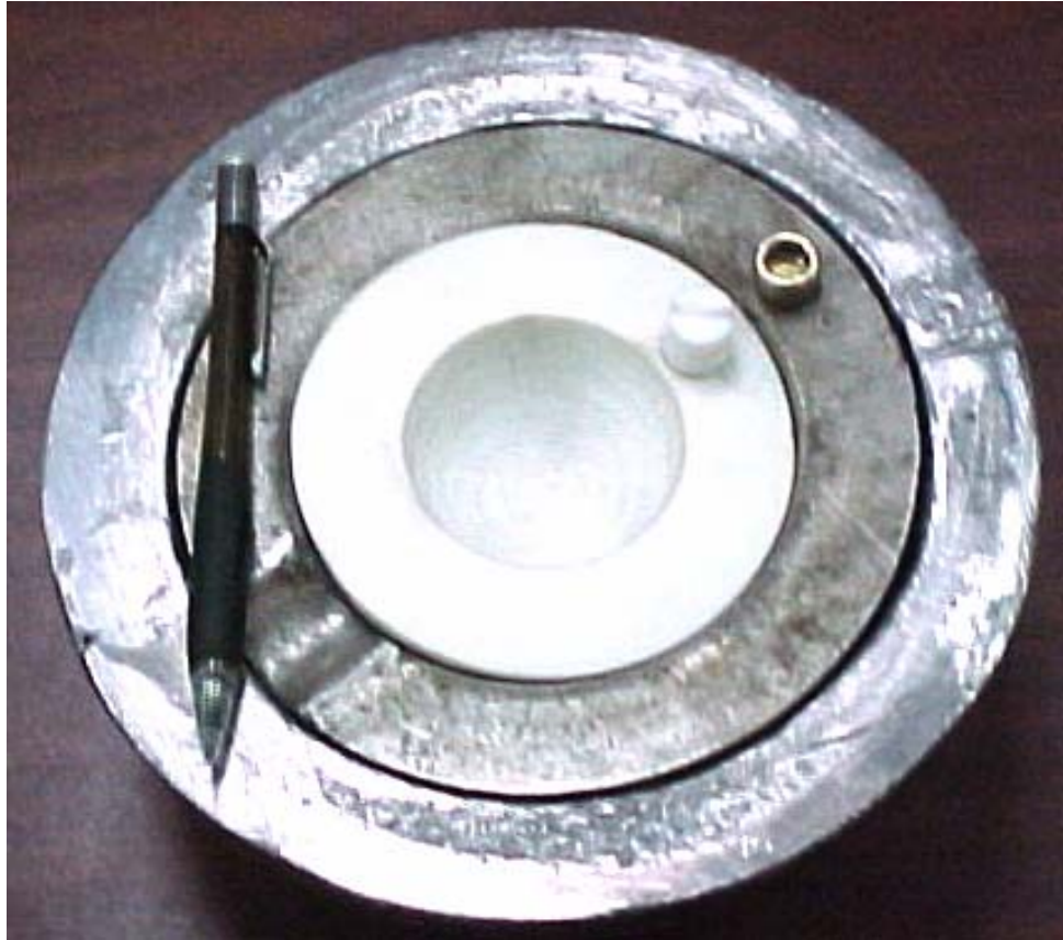
Figure 5 Components of a weapon mock-up consisted of an inner polymer bowl containing a distributed source, a simulated reflector made of spun aluminum filled with water, and a simulated lead tamper on the outside
