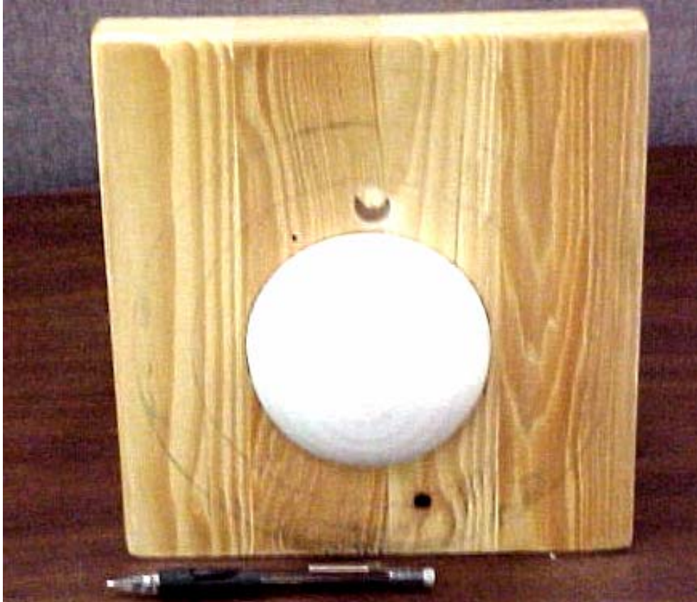
Figure 39 Distributed Cs-137 bowl source in testing configuration
