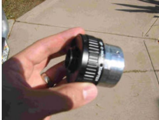
Figure 37. C-Mount Adapter for the Merlin Camera
