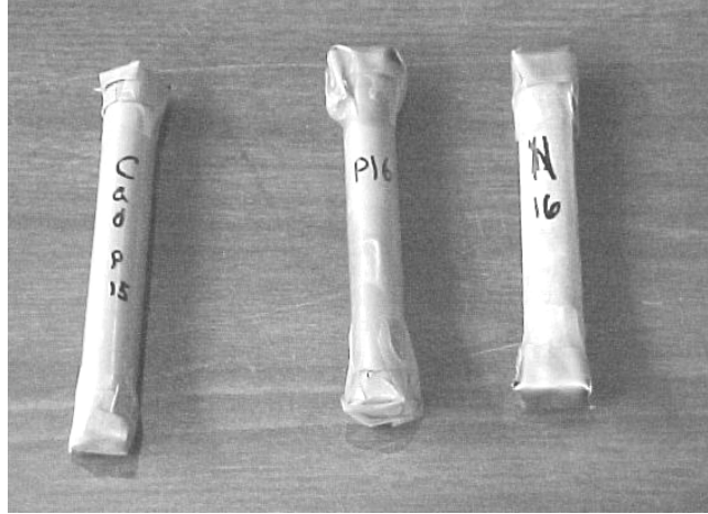
Figure 20: Containers wrapped in cadmium. Cadmium's high thermal neutron cross section helps to minimize activation of the samples.
