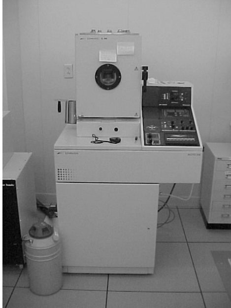
Figure 8: E-Beam Deposition System. This system deposited the metal contacts onto the samples
