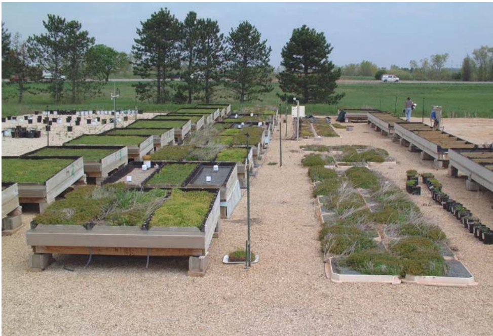
Figure 4.41 Test Platforms. Model-scale platforms used for evaluating storm water retention. (VanWoert et al., 2003)
