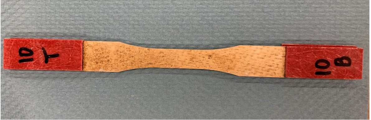
Figure 8. Specimen equipped with tabs and ready for testing
