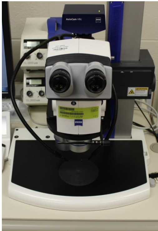
Figure 15. Zeiss Discovery V12 optical microscope equipped with an AxioCam HRc digital camera
