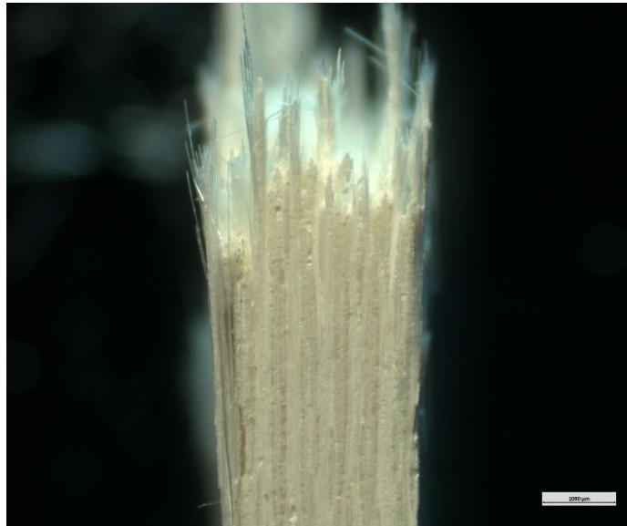
Figure 79. Optical micrograph of the fracture surface of N720/AM specimen tested in tension-tension fatigue at 1200°C in steam. \sigma_{\max} = 60 MPa, N_f > 100000 .
