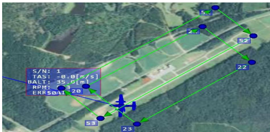
Figure 3. Waypoint locations Attack Flight Plans (Carnahan & Heiges, 2015)
