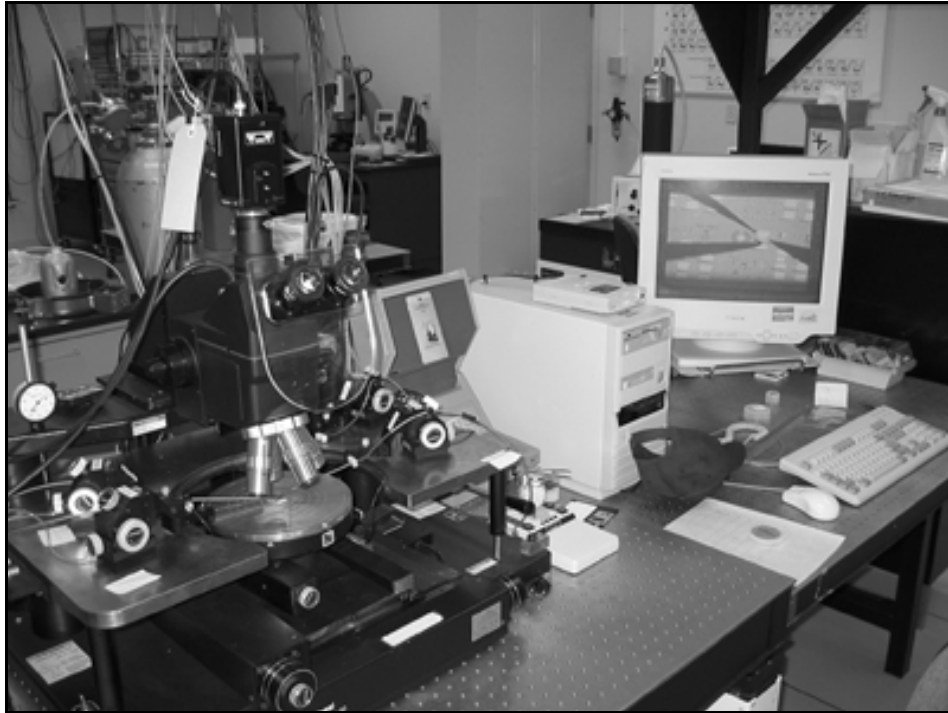
Figure 25. AFIT Probe-Stand Used for Pre- and Post-Irradiation I - V Characterization
