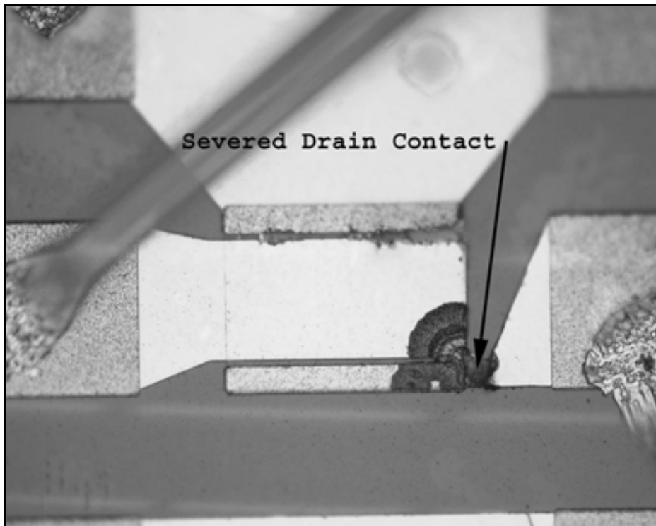
Figure 63. Sample A0315 FatFET Irradiation Experiment Drain Damage
