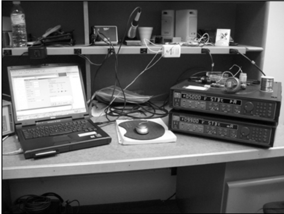
Figure 23. Building 470 Experimental Setup for Pre-Irradiation I - V Characterization
