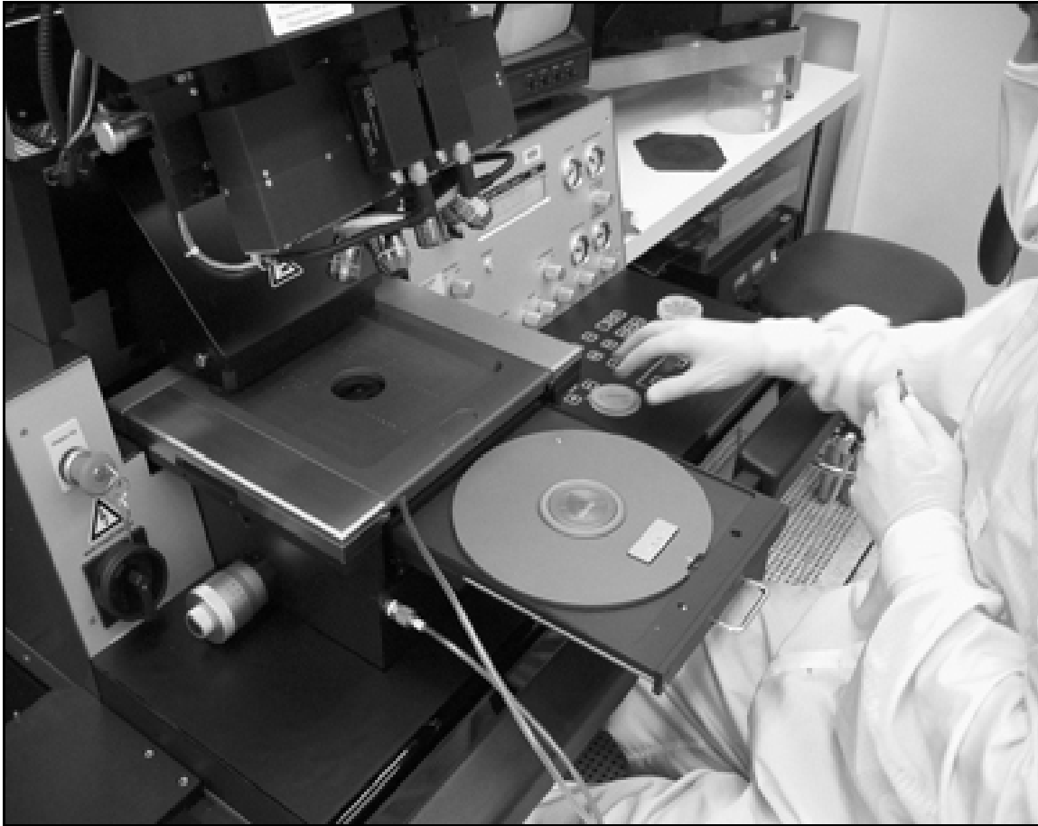
Figure 15. AFRL/SNDD UV Exposure System Used for Photolithography
