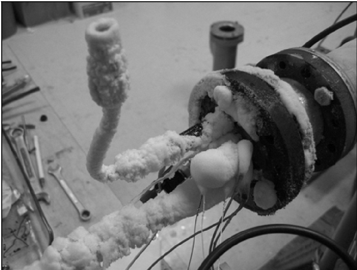
Figure 31. Cold Head Operation Under Cryogenic Conditions
