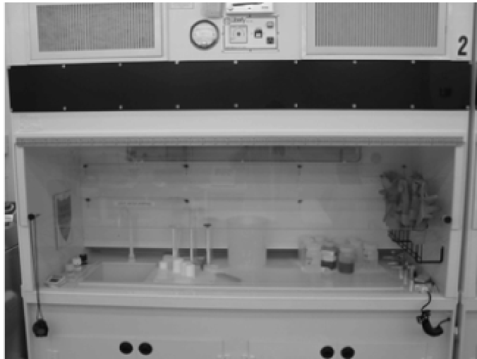
Figure 6.1: A photo graph of the clean room acid chemical station, with a venting hood.
