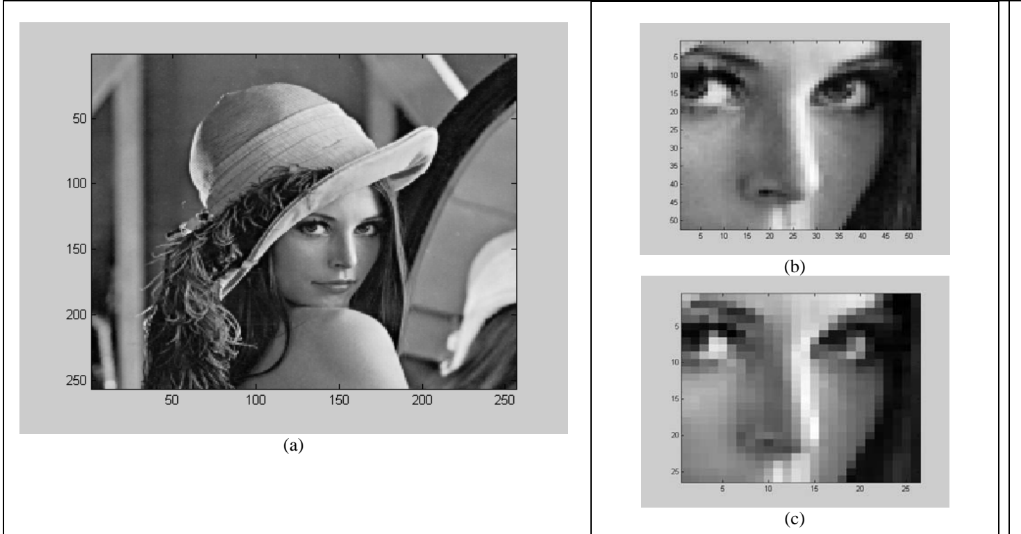
Figure 30 Lenna image (a) with the interpolated portion boxed, (b) with this portion enlarged, (c) with this portion low pass filtered and down sampled.
