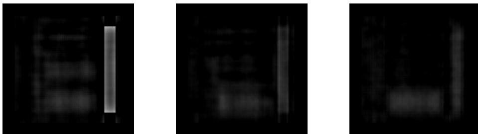
Figure 47 Bands 5, 6, and 7 are shown here from left to right. Bleeding from sources located in nearby frequency bands is shown in each image. The bleeding gets stronger as the image gets closer to that particular source location.
