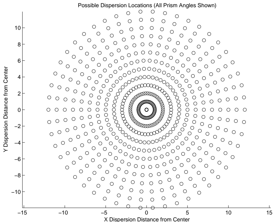
Figure 10 Any pixel location of the object cube can be dispersed at a distance from the origin represented by the circles shown here. The center of the pattern represents a shift distance and direction of zero.
