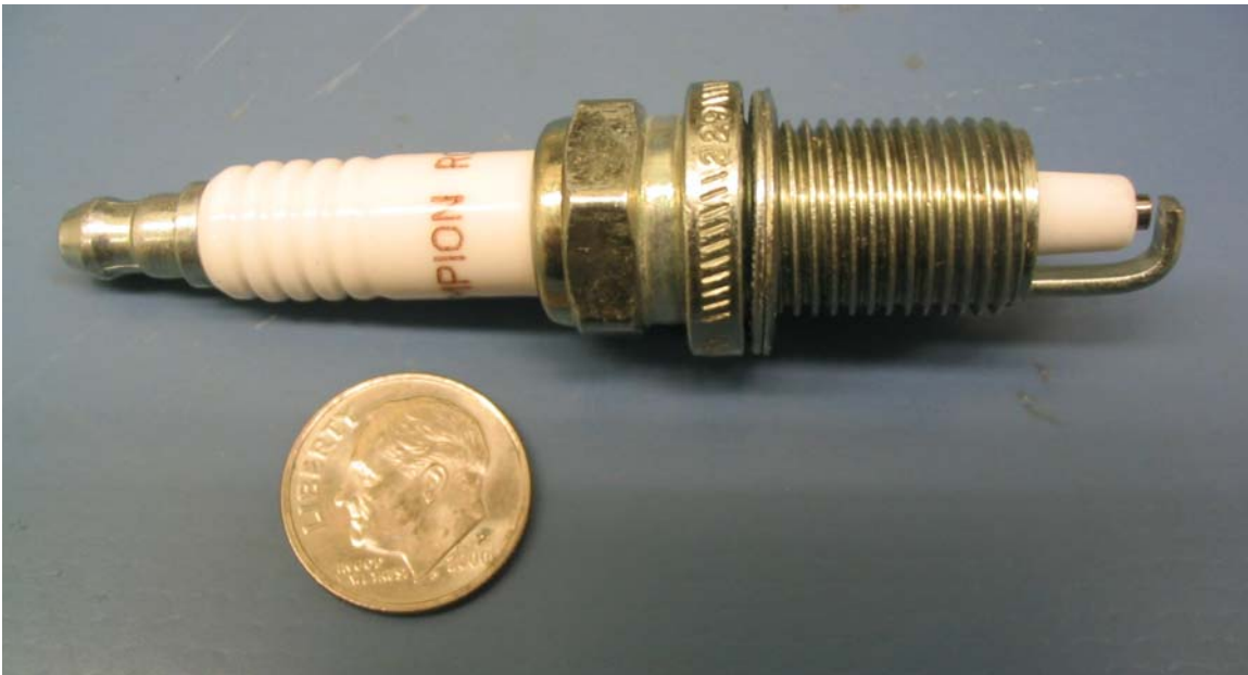
Figure 3. Champion RC12LYC Spark Plug
