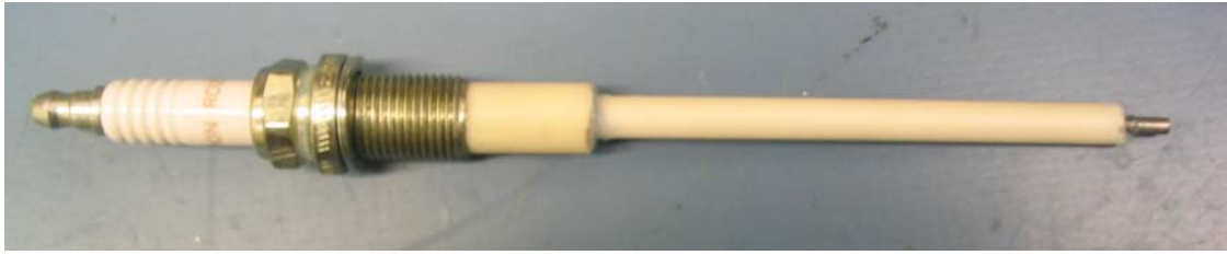
Figure 6. Long Probe with 10.16 cm insulated extension
