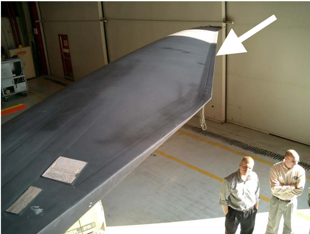
Figure 14. Trim tab on blade of AH-64 Apache
