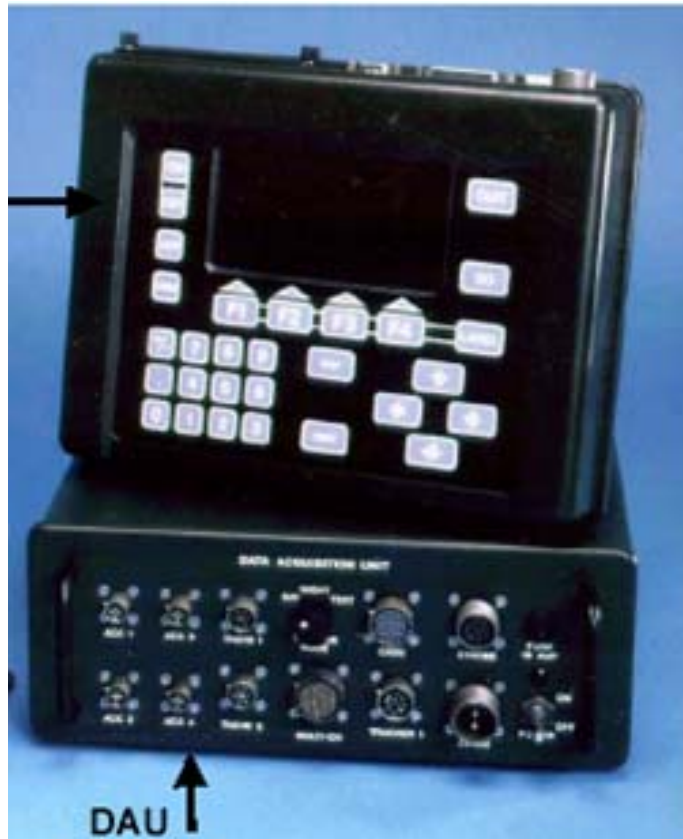
Figure 7. Data acquisition unit and user interface [AVATM, 2-1]
