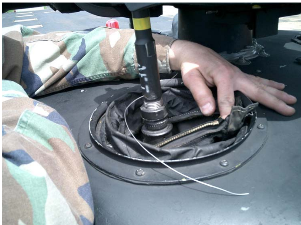
Figure 28. Pitch link lock on CH-47 Chinook
