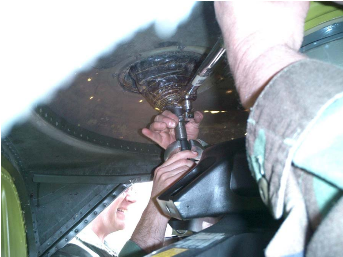
Figure 27. Pitch link adjustment on CH-47 Chinook
