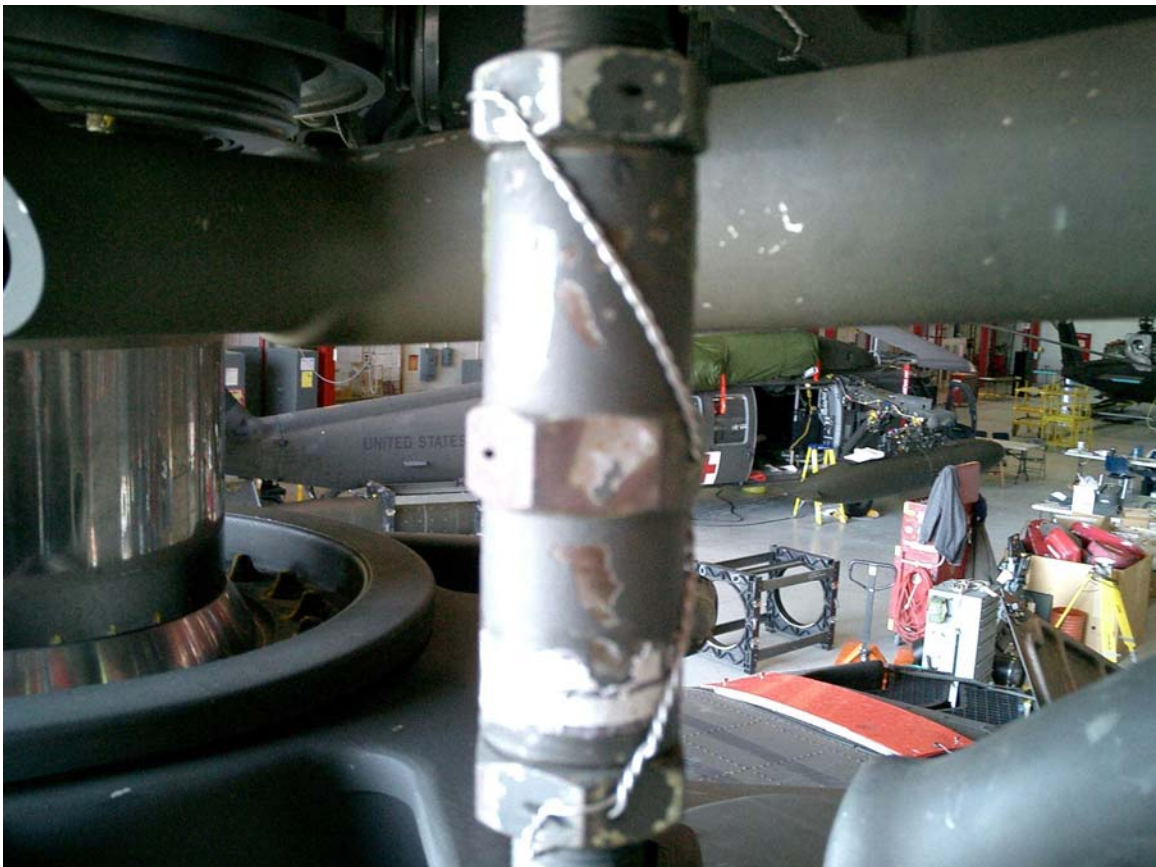
Figure 30. U.S. Army AH-64 Apache adjustable pitch link design accidentally rotate the pitch link turnbuckle the wrong way, leading to smoothing failure. [Bale, 2004] Proper training can help reduce the chance of mechanic error. Figure 30
