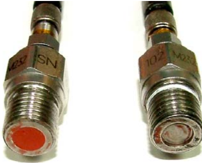
Figure 3-3: PCB Pressure Transducers with and without RTV Silicone coating
