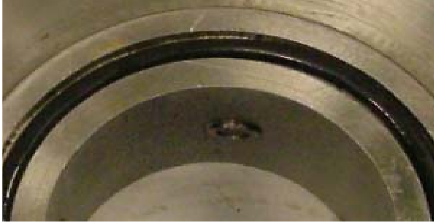
Figure 3-7: PCB Transducer protruding into shock tube
