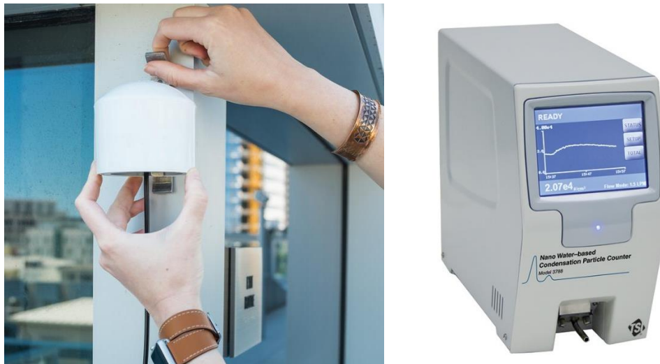
Figure 9. A PurpleAir sensor can be discreetly installed (PurpleAir, 2020) (Left), the TSI 3788 is capable of 2.5-nm particle detection (TSI, 2018) (Right)
