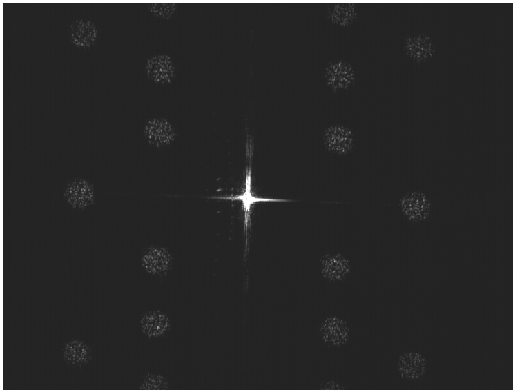
Figure 4.25: Phase Hologram vs Phase Grating: The far field image created with a phase hologram loses intensity in each beam but all 18 original beams are present and remain focussed. (The brightness and contrast levels of this picture have been enhanced by 15% for printing of this document).
