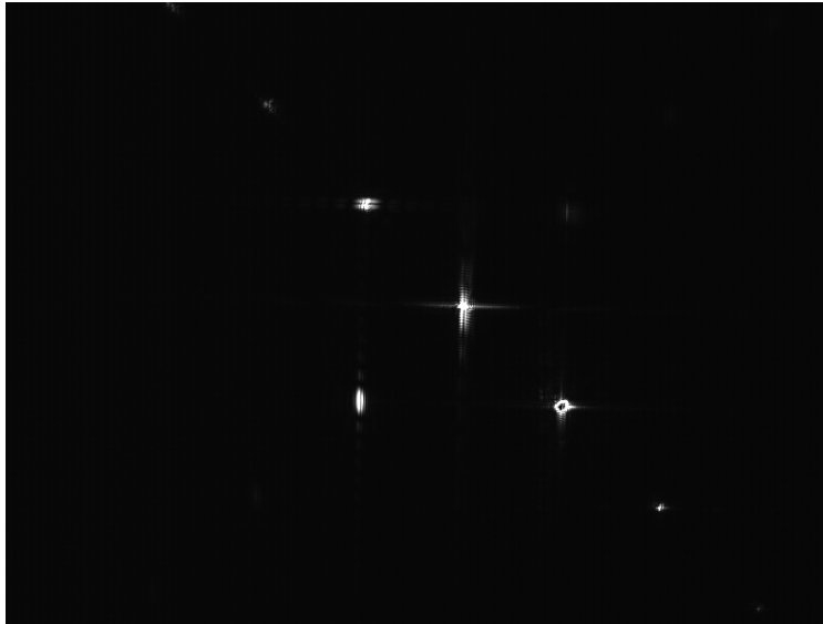
Figure 4.7: Intensity variation: The original beam is split into four beams of varying intensity. The upper and lower left beams are at an equal medium power, the upper right beam is turned off, and the lower right beam contains the most intensity - saturating the camera in this case. SLM limitations cause some residual light to remain in the zeroth order and also to be steered to the second order.
