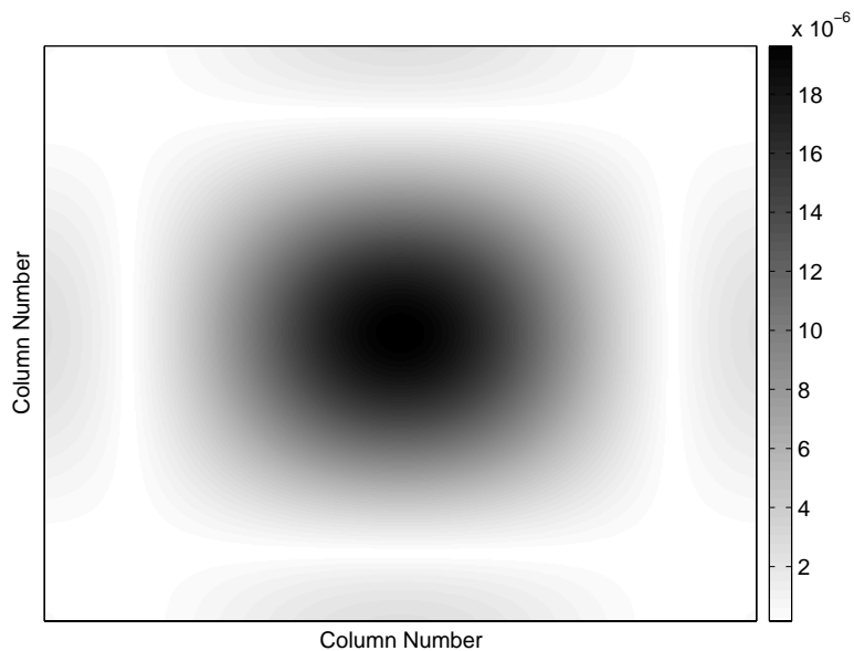
Figure 3.5 Cross Temporal Matrix (CTM) for Downconverting Channelized Receiver Data, No Noise Present
