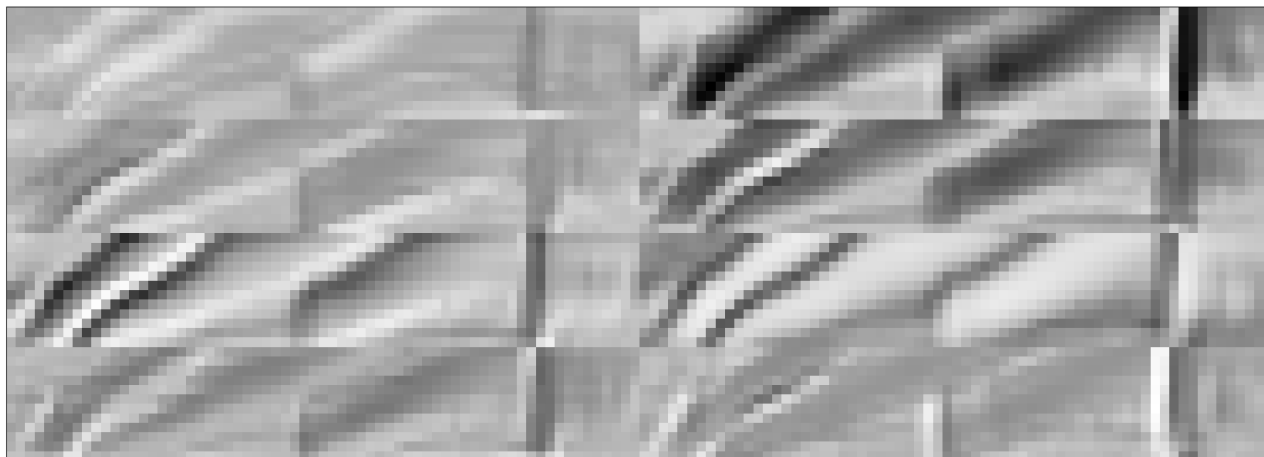
Fig. 6. Feature maps for the “crossing” in the second convolutional layer of the neural network
