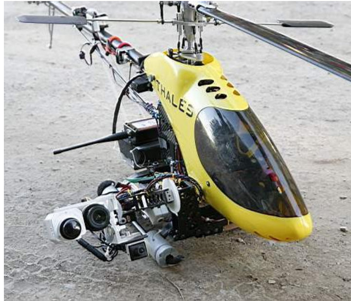
Figure 7. UAV platform with sensory payload consisting of 3 cameras; high-resolution, low-resolution and thermal
