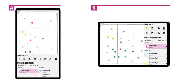
Fig. 3.24 The Selection List (*a*) opens on the bottom part of the screen if the device is in portrait mode, and it occupies the (*b*) right part of the screen in landscape mode.
