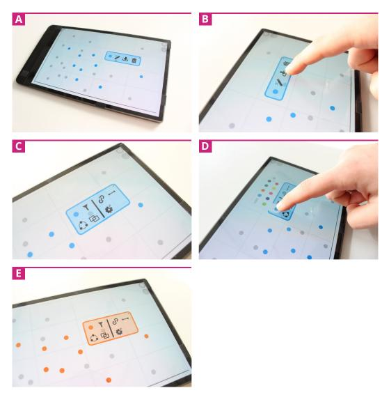
**Fig. 4.3** (*a*) The Selection Menu for a temporary selection in novice mode. (*b*) Pressing the icon to store the selection and make it permanent. (*c*) The Selection Menu for the newly created permanent selection. (*d*) Pressing the color icon to pick another color. (*e*) The Selection Menu after the color change.
