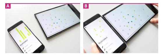
**Fig. 4.5** (*a*) The Detail View contains an visual representation of the selection that shows the visualization it was originally created from, here a bar chart. (*b*) When positioned next to a Visualization View, this visual representation adjusts to match the Visualization View's visualization type, in this case it turns to a scatter plot.
