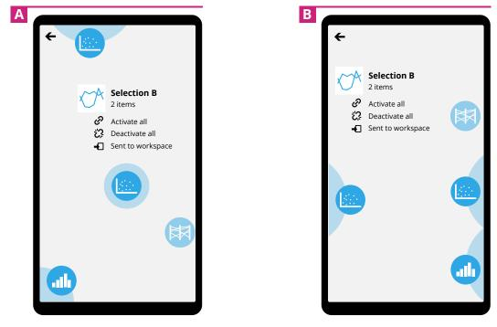
**Fig. 3.39** The two versions of the Portal View: (*a*) on spatially aware devices and (*b*) on spatially agnostic devices. (*a*) The portals for the devices are positioned around the edges using spatial information. The portal for the Visualization View located on the same device is positioned in the view's center. (*b*) The portals for the devices are positioned on the right side of the screen. The portal for the Visualization View located on the same device is positioned on the left side.
