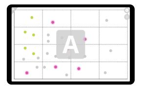
**Fig. 3.6** A device showing the overlay that appears when the user highlights the devices belonging to the workspace by shaking the device. The overlay shows the letter that corresponds to the workspace.
