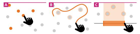
Fig. 3.4 Methods for selecting items or areas in a visualization: (*a*) Tapping to select items, (*b*) drawing a Lasso to select items, and (*c*) Brushing over an axis to select a range.
