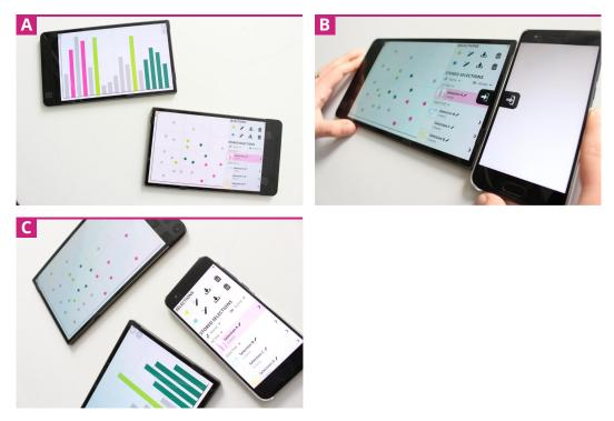
**Fig. 4.4** (*a*) Two Visualization Views where one of them shows the Selection List on screen. (*b*) Putting another device beside it, shows the Edge Menu with the option to transfer the Selection List. (*c*) The transferred Selection List on a separate device.
