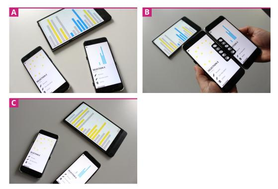
Fig. 4.6 (a) A Visualization View showing a bar chart with two selections and the Detail Views of those. (b) Juxtaposing the Detail Views shows the Edge Menu with possible Join Operations. (c) The final setting after choosing to create the union of the two selections.
