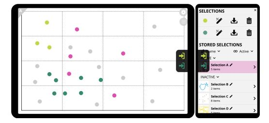
**Fig. 3.27** Edge Menu for a Selection List is side-by-side to a Visualization View. It includes a *Store selection* button for every temporary selection in the Visualization View. In this case two buttons for a green selection and a blue selection.
