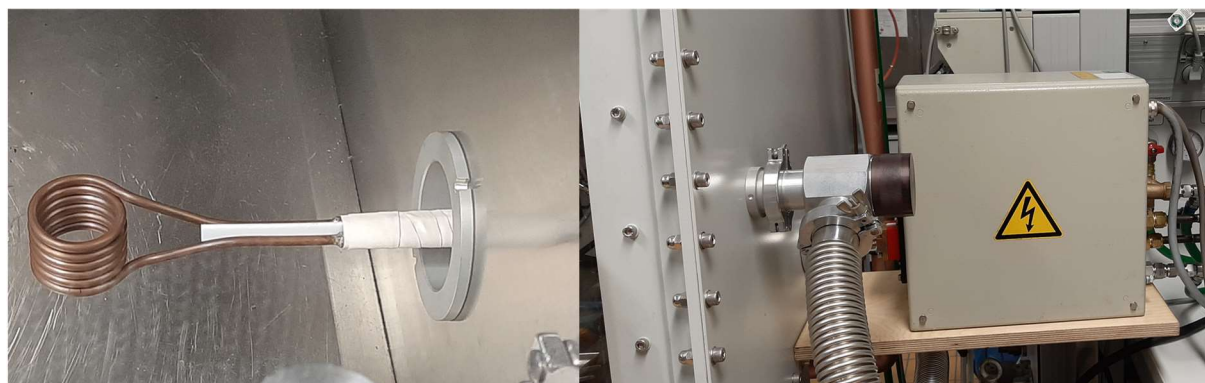
Figure 3.2. The experimental setup of induction melting present inside the glove box.
