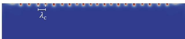
Fig. 7. Evolving patterns of cracks nucleation in the specimen ( \Delta T = 1000 K; l_G = 0.15l , \sqrt{l_G l} = 0.005 mm, \lambda_c \approx 0.06 mm).
