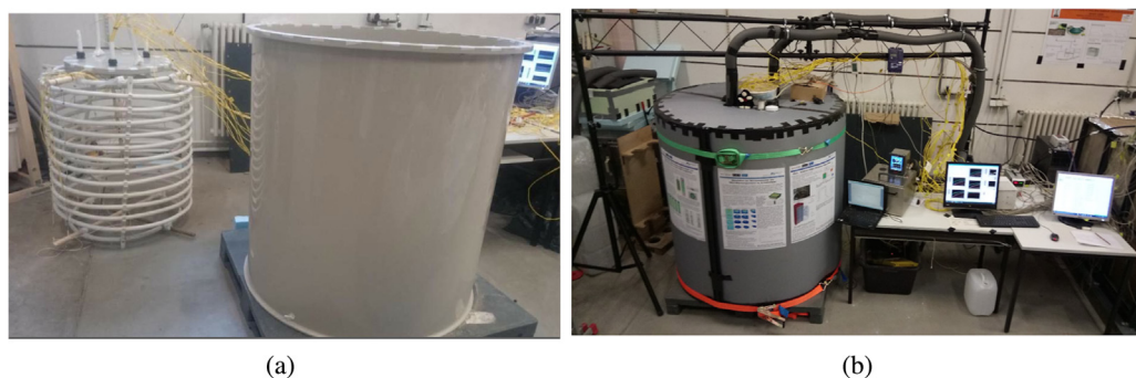
Fig. 9. Configuration of the SHS used in IGLU TES: (a) a heat exchanger and a cylindrical mold prepared for the SHS; (b) a single configured testing module. Images with kind permission by Prof. Frank Wuttke, Chair of Geomechanics & Geotechnics, Kiel University, www.geotechnics.ifg.uni-kiel.de .
