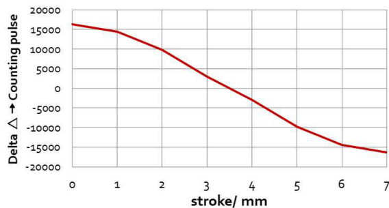
Figure 12: Signal quality above stroke area in case 2 solenoid coils are used
