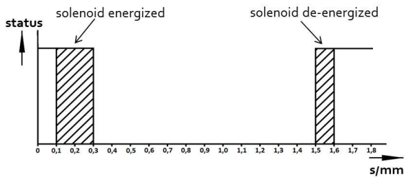
Figure 9: Optimized position detection
