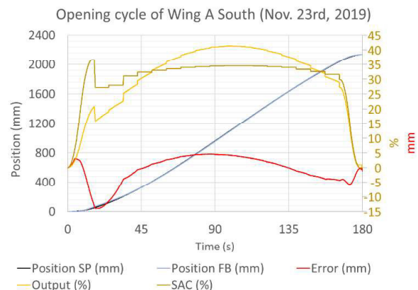
Figure 20: Pre-commissioning results on wing A South.
