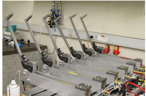
Figure 4: Picture of endurance test with six clamps.
